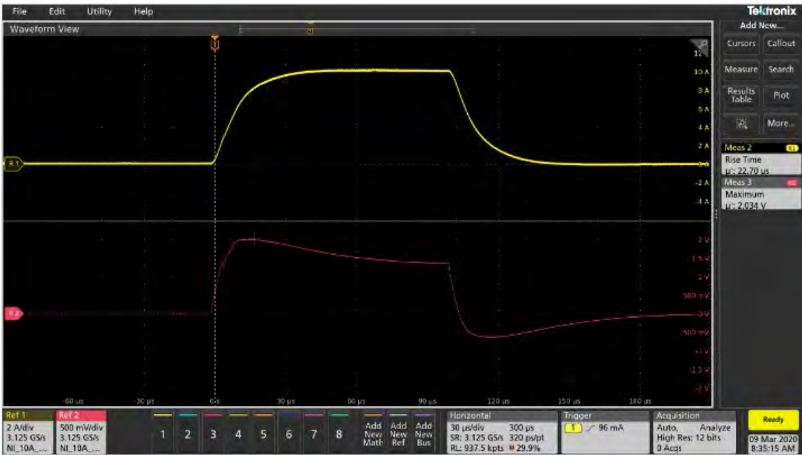
Figure 6. 22 \mu s rise time 10 A Pulse on inductor 1 \mu H
