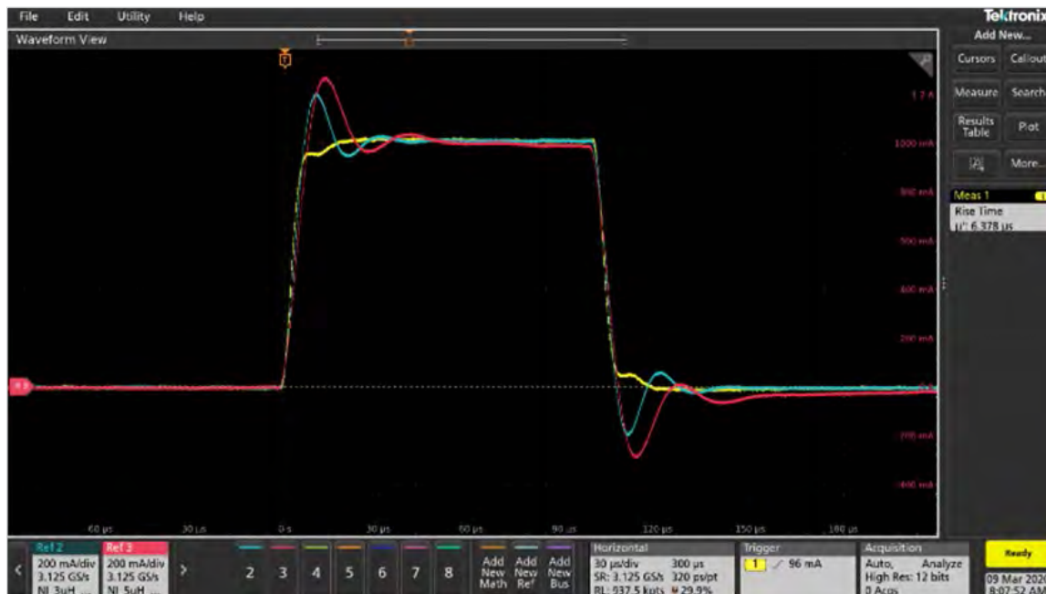
Figure 5. 1 A 100 \mu s Pulses on inductors, 1 \mu H (yellow), 3 \mu H (blue), and 5 \mu H (red).
