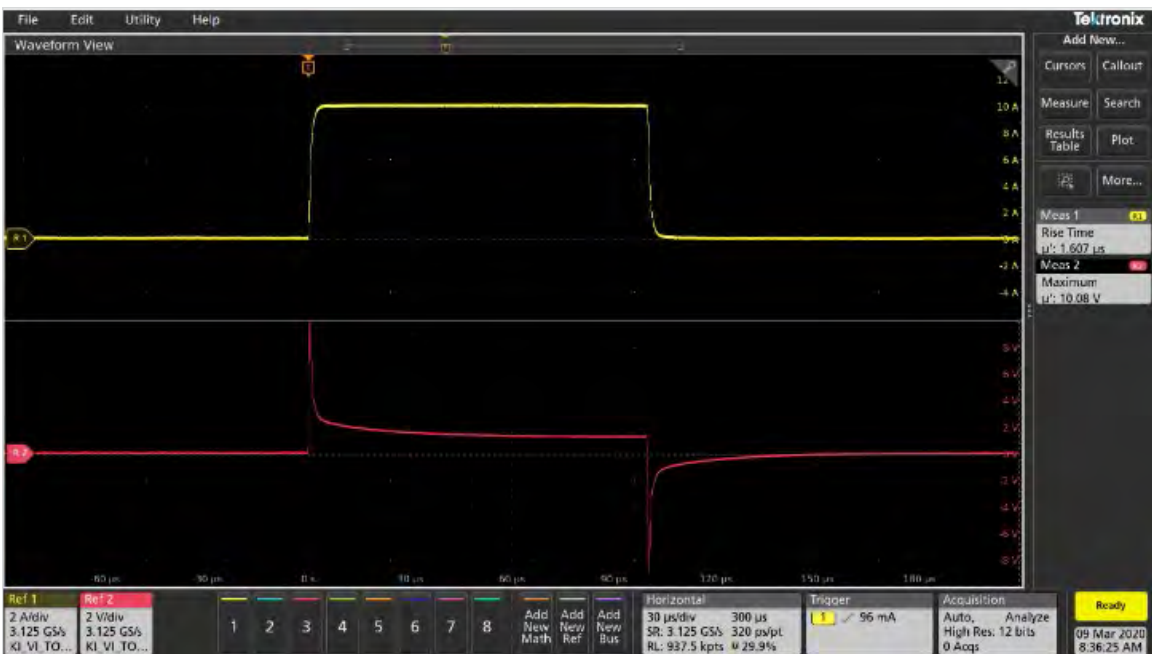
Figure 7. 1.6 \mu s rise time 10 A Pulse on inductor 1 \mu H
